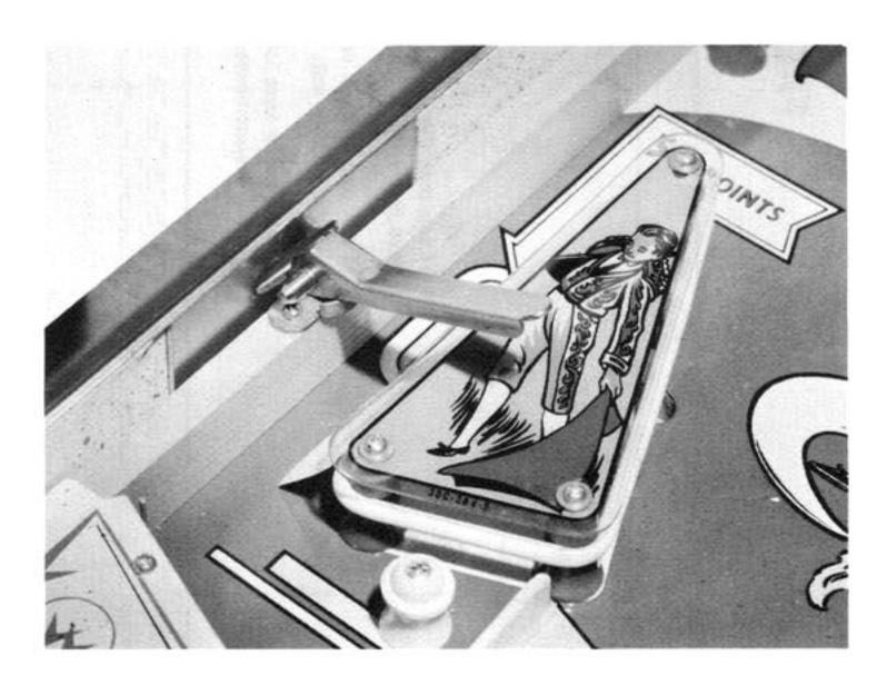
4. TO RELOCK, LOWER PLAYBOARD INTO CABINET. SLIDE PLAYBOARD TO FRONT OF CABINET AND REVERSE THE ABOVE PROCEDURE.
