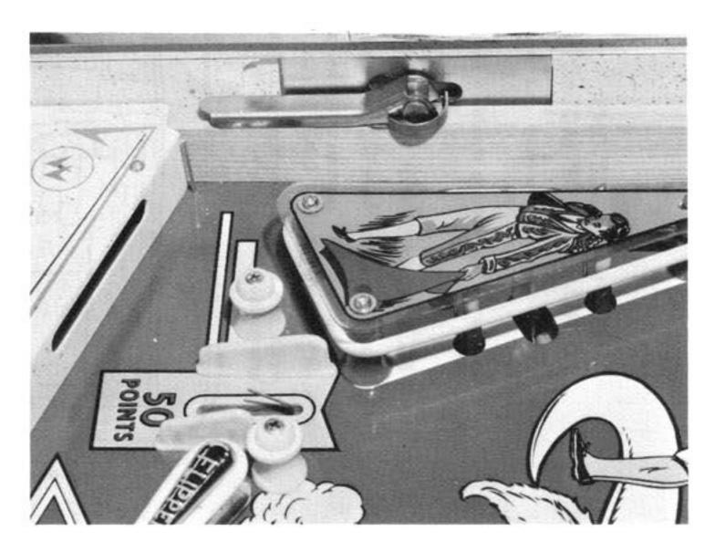
2. TO UNLOCK PLAYBOARD LIFT LOCK HANDLES AS SHOWN
